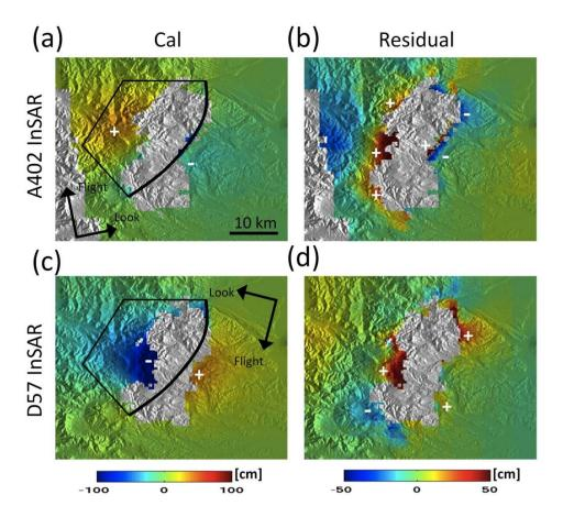
Figure 2-5: (a) Calculated InSAR data for the ascending track 402 from the fault model in Figure 2-4 and (b) misfit residuals from the observed one in Figure 2-2c. (c) Calculated InSAR data for the descending track 57 from the fault model in Figure 2-4 and (d) misfit residuals from the observed one in Figure 2-2d.
