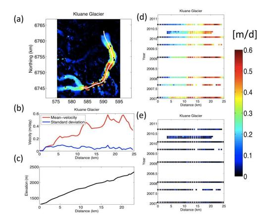
Figure 3-32: Surface velocity evolution at Kluane Glacier. (a) Spatial surface velocity and the flow line. Horizontal and vertical axes are UTM coordinates. (b) Mean-velocity profile of the data and the standard deviation along the chosen flow line at (a). (c) The elevation profile along the chosen flow line at (a). (d) Spatial—temporal evolution of the surface velocities recorded from 2006 to 2010. (e) Error estimates of (d).
