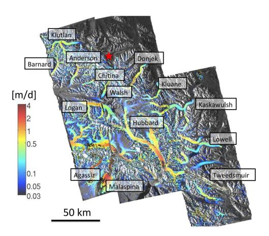
Figure 3-6: Surface velocity map derived from three paths of ALOS/PALSAR. Please note the color scale is shown as logarithm. Red star indicates the location of Trapridge Glacier, whose size is too small to image from Satellite data.
