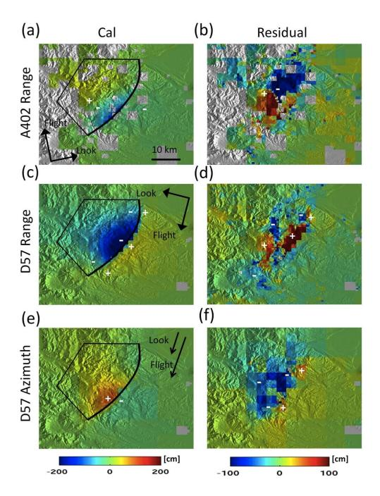
Figure 2-6: (a) Calculated range-offset data for the ascending track 402 from the fault model in Figure 2-4 and (b) misfit residuals from the observed one in Figure 2-2e. (c) Calculated range-offset data for the descending track 57 from the fault model in Figure 2-4 and (d) misfit residuals from the observed one in Figure 2-2f. (e) Calculated azimuth offset data for the descending track 57 from the fault model in Figure 2-4 and (f) misfit residuals from the observed one in Figure 2-2h.
