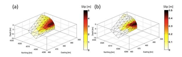
Figure 2-4: Geometry and slip distribution of a west-dipping fault model inferred from GPS data alone. (a) Dip-slip component and (b) left-lateral slip component. Note the difference in the scale of the color bars.
