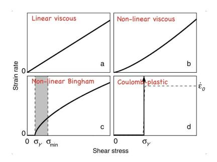
Figure 3-37: Stress-strain rate relations for modeled till flow laws (Kavanaugh and Clarke, 2006). (a) Linear-viscous till. (b) Nonlinear-viscous till (c) Nonlinear-Bingham till. Shaded region represents transition zone between elastic ( $\tau < \sigma_Y$ ) and viscous ( $\tau > \sigma_{min}$ ) behaviors. (d) Coulomb-plastic till (solid line) and hyperbolic tangent approximation of Coulomb-plastic behavior.  $\varepsilon_0$  stands for the reference strain rate.
