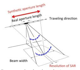
Figure 1-1: Geometry of real and synthetic aperture radar.
