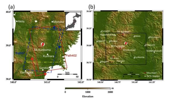
Figure 2-1: (a) Studied area of the Iwate-Miyagi inland earthquake and nearby cities, and the observed areas by ALOS/PALSAR (solid and dashed boxes). Solid and dashed boxes represent ascending and descending orbits, respectively. (b) Expanded area of the dash—dot box in part (a). Locations of major mountains and GPS stations near the epicenter are shown. The solid box indicates the area in Figure 2-2.
