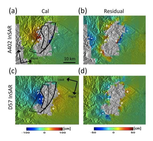
Figure 2-9: (a) Calculated InSAR data for the ascending track 402 from the fault model in Figure 2-11 and (b) misfit residuals from the observed one in Figure 2-2c. (c) Calculated InSAR data for the descending track 57 from the fault model in Figure 2-11 and (d) misfit residuals from the observed one in Figure 2-2d. Plan view of the fault model in Figure 2-11 is also indicated by a black line with the thick lines representing the top edge.
