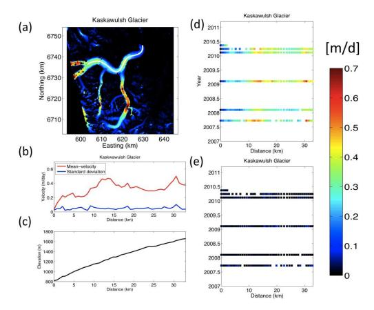
Figure 3-31: Surface velocity evolution at Kaskawulsh Glacier. (a) Spatial surface velocity and the flow line. Horizontal and vertical axes are UTM coordinates. (b) Mean-velocity profile of the data and the standard deviation along the chosen flow line at (a). (c) The elevation profile along the chosen flow line at (a). (d) Spatial—temporal evolution of the surface velocities recorded from 2007 to 2010. (e) Error estimates of (d).
