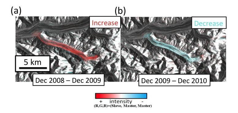
Figure 3-13: (a) RGB composite intensity image of an old image obtained on December 23, 2008 and a new image obtained on December 26, 2009. Red-colored area indicates an increase in the scattering intensity. (b) The composite image of an old image obtained on December 26, 2009 and a new image obtained on December 29, 2010. Cyan-colored area indicates a reduction in the scattering intensity.
