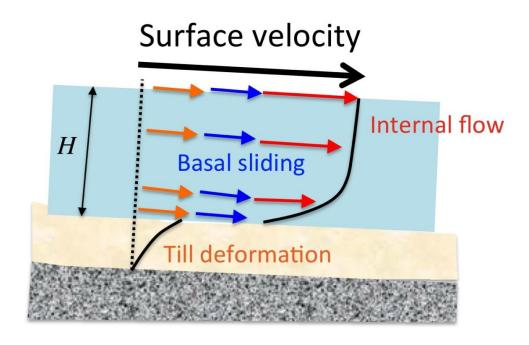
Figure 3-3: The three components of the surface velocity.
