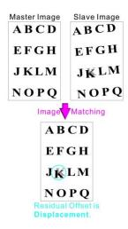
Figure 1-2: Images of pixel offset technique. After co-registration of two images, the local offsets are detected as displacements.
