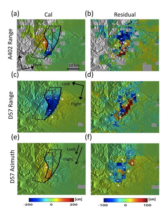
Figure 2-10: (a) Calculated range-offset data for the ascending track 402 from the fault model in Figure 2-12 and (b) misfit residuals from the observed one in Figure 2-2e. (c) Calculated range-offset data for the descending track 57 from the fault model in Figure 2-11 and (d) misfit residuals from the observed one in Figure 2-2f. (e) Calculated azimuth offset data for the descending track 57 from the fault model in Figure 2-11 and (f) misfit residuals from the observed one in Figure 2-2h.
