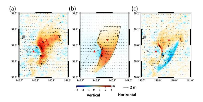
Figure 2-13. (a) Observed 3D displacements derived from the SAR data by Ando and Okuyama (2010). Vectors represent horizontal displacements, and colors represent vertical displacements. (b) Calculated 3D displacements, based on the source model in Figure 2-12. (c) Misfit residuals from the observed 3D displacements. The star and triangle indicate the epicenter and Mt. Kurikoma, respectively. The black dot indicates the GPS station, Kurikoma2.
