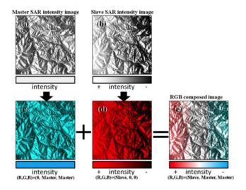
Figure 1-3: Principle of the RGB (red, green, and blue) method (Yasuda and Furuya, 2013). (a) Old radar scattering intensity image. (b) New intensity image. (c) Old intensity image marked with cyan. (d) Newer intensity image marked with red. (e) Composite image after the RGB addition of the intensity images in (c) and (d). While the red/cyan areas show where the surface scattering intensities have increased/decreased, areas that underwent no intensity changes remain gray.
