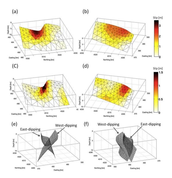
Figure 2-11: Geometry and slip distribution of the east-dipping (F1) and west-dipping (F2) segment model inferred from GPS and SAR data. (a) Dip-slip component for F1, (b) dip-slip component for F2, (c) left-lateral slip component for F1, and (d) left-lateral slip component for F2. Note the difference in the scale of the color bars. (e,f) 3D perspective of the fault geometry viewed from (e) SSW and (f) NNE.
