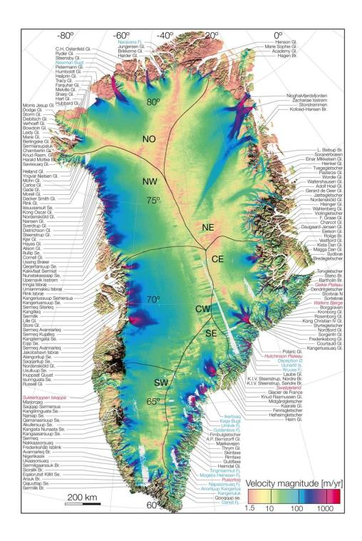
Figure 3-2: Ice velocity map of the Greenland Ice Sheet derived from satellite radar interferometry data from ALOS PALSAR, Envisat ASAR and RADARSAT-1 (Rignot and Mouginot, 2012)
