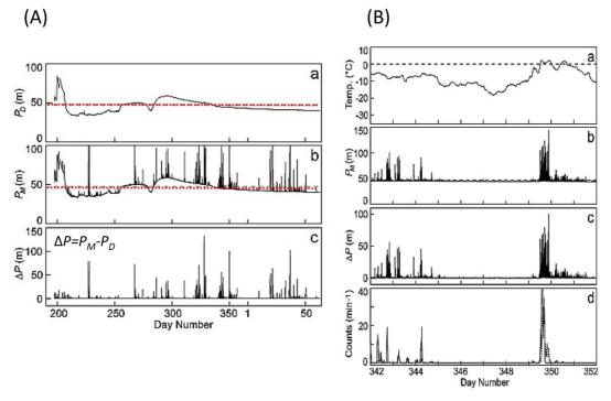
Figure 3-36: Basal water pressure changes at Trapridge Glacier (After Kavanaugh, 2009). (A) Water pressure changes from July 16 2005 to March 4 2006 (a) Discrete pressure record (b) Maximum pressure record. Red dashed lines indicate flotation value (c) the difference (b)-(a). (B) Data from 8 to 18 December, 2005 (a) Temperature (b) Maximum pressure record (c) the difference between (c) - Discrete pressure record. (d) A number of icequake events.
