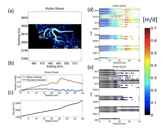
Figure 3-30: Surface velocity evolution at Klutlan Glacier. (a) Spatial surface velocity and the flow line. Horizontal and vertical axes are UTM coordinates. (b) Mean-velocity profile of the data and the standard deviation along the chosen flow line at (a). (c) The elevation profile along the chosen flow line at (a). (d) Spatial—temporal evolution of the surface velocities recorded from 2007 to 2011. (e) Error estimates of (d).
