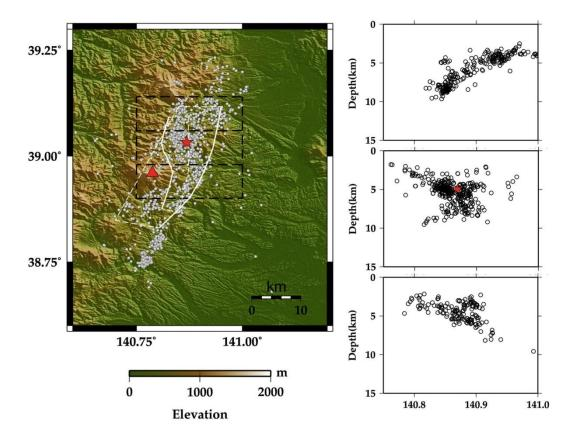
Figure 2-7: (Left) Plan view of the aftershocks and (right) their three cross sections from the north to the south. The white lines indicate the location of the two-segment model inferred from GPS and SAR data; the geometry and slip distribution are shown in Figure 2-11. The thick lines indicate the top edge of our fault model. The star and triangle indicate the epicenter and Mt. Kurikoma, respectively.
