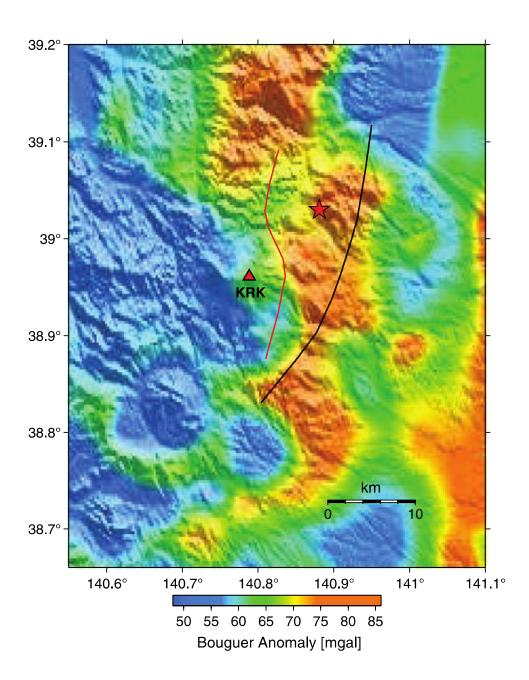
Figure 2-14: Bouguer gravity anomaly and the location of the two-segment fault model. The black and red lines indicate the top edge of the west- and east-dipping fault models, respectively. KRK stands for Mt. Kurikoma. The star indicates the epicenter.
