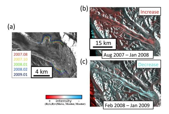
Figure 3-11: (a) Terminus advances at the Tweedsmuir Glacier recorded from ALOS/PALSAR intensity images. (b) RGB composite intensity image of an old image obtained on August 29, 2007 and a new image obtained on January 14, 2008. Red-colored area indicates an increase in the scattering intensity. (c) The composite image of an old image obtained on February 29, 2008 and a new image obtained on January 16, 2009. Cyan-colored area indicates a reduction in the scattering intensity.
