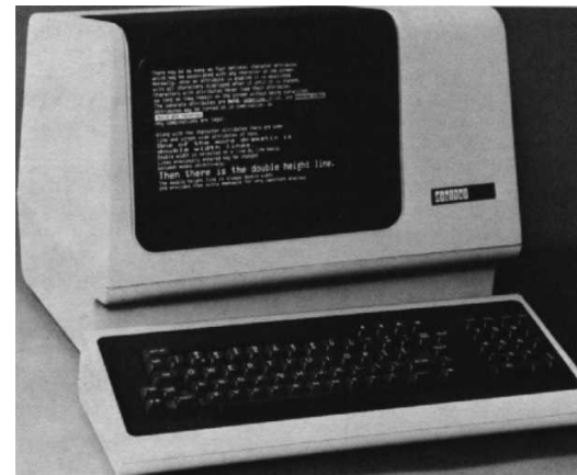
Digital's VT100 video terminal (1978) http://vt100.net/
