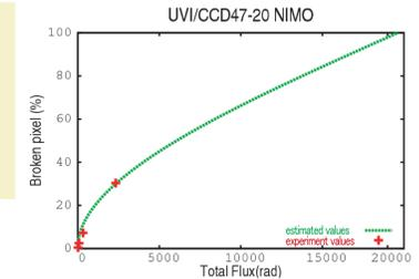
Fig.5.2: Relation between total dose and dark spikes of CCD47-20 NIMO. The presumed curve is estimated by probability calculation, and fitted with experient values. Under 10 krad(s) total dose, it is expected that the half pixel of CCD receive some damages..
