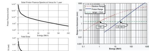
Fig.5.5: Ranges of electron and proton in aluminum. With about 3mm aluminum, CCD can be shielded from the proton of 25MeV.
