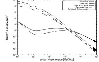
Fig.5.4: The proton flux around Venus which is estimated using the CREME model. At the time of a flare event, it is monotonous reduction as it becomes high energy. At the time of quiet time, it has an extremum near GeV energy.
