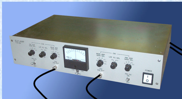
ELF Main Amplifier (Gain/6-66 dB, Notch Fil./50,100,150 Hz)
