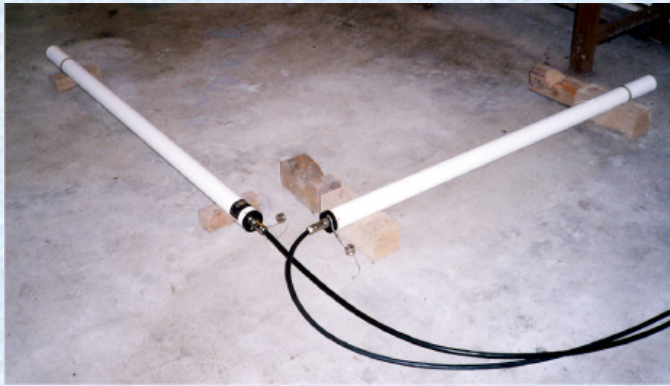
Search Coil Magnetometers (0.3 mV/pT @1-400 Hz)
