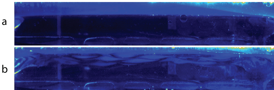
FIGURE 1. Cross-section of the experimental tank containing the optical image (arbitrary colors) a) initial, stable condition, b) two-layer convection.
