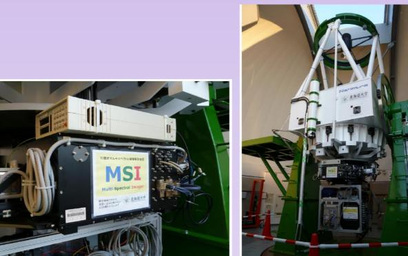
Fig. 2 The 1.6 m Pirka telescope and Multi-Spectral Imager (MSI)
