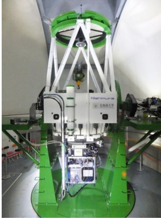
Figure 2.3: Picture of the 1.6-m Pirka telescope.
